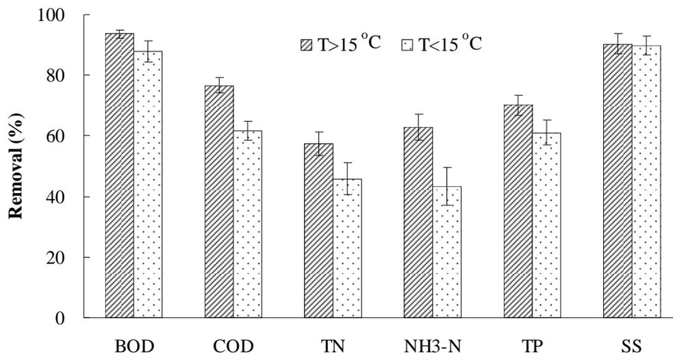
**Figure 4** Comparison of pollutants removals by CW system in high water temperature and low water temperature periods
