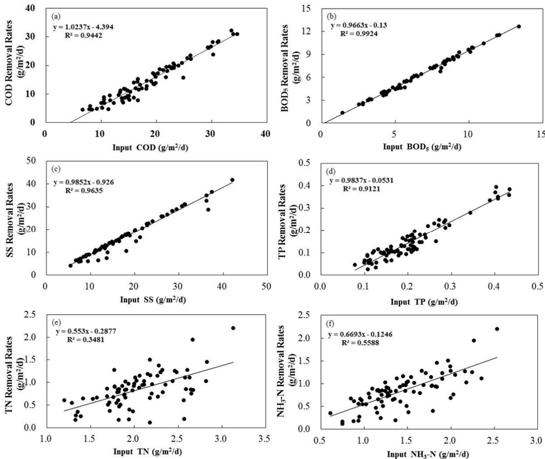
**Figure 3** Correlation charts between input loading and removal rates for: (a) COD; (b) BOD<sub>5</sub>; (c) SS; (d) TP; (e) TN; (f) NH<sub>3</sub>-N
