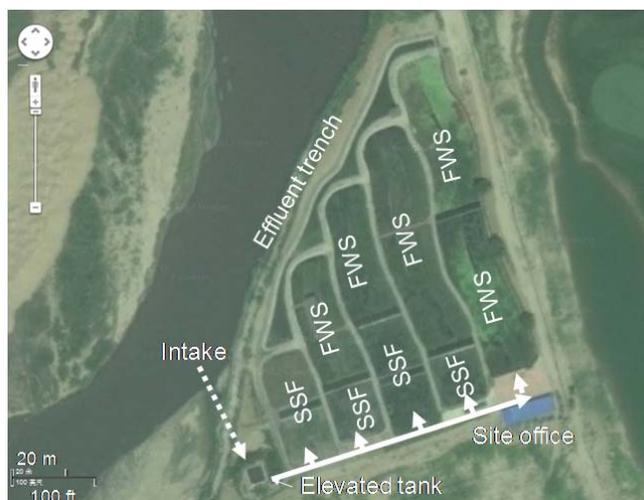
**Figure 1** Satellite view of the pilot constructed wetland (CWs) system
