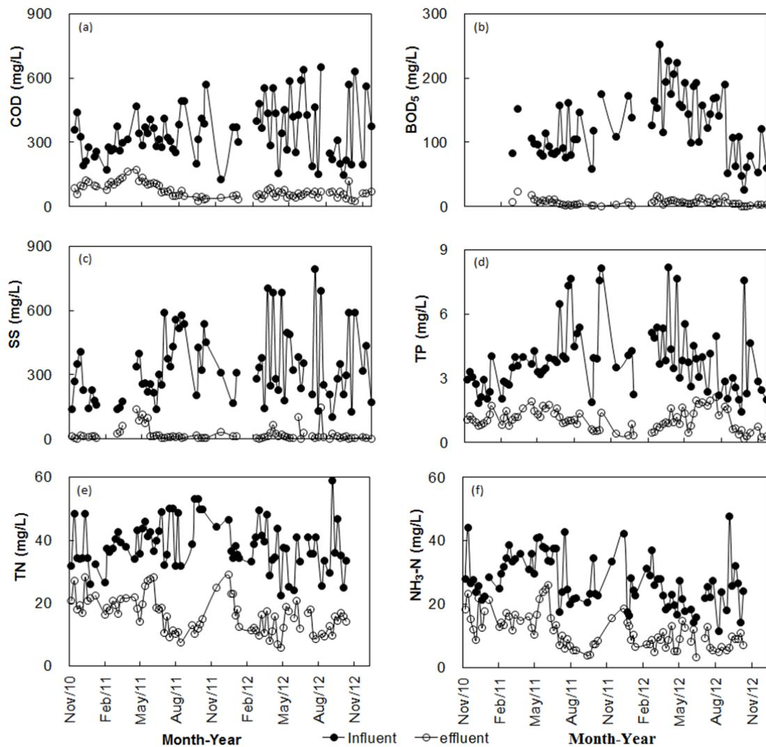
**Figure 2** Concentrations of: (a) COD; (b) BOD<sub>5</sub>; (c) SS; (d) TP; (e) TN; (f) NH<sub>3</sub>-N in the pilot CW system during the experimental period
